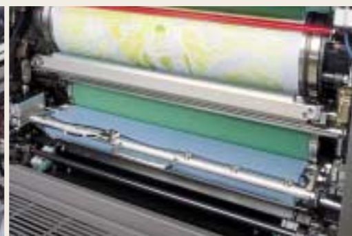
Automatic blanket cleaning device
